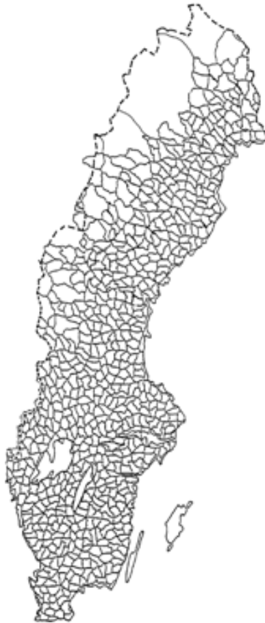
Figure 1. The extent of the third precise levelling network of Sweden (Lantmäteriet, 2009a)
