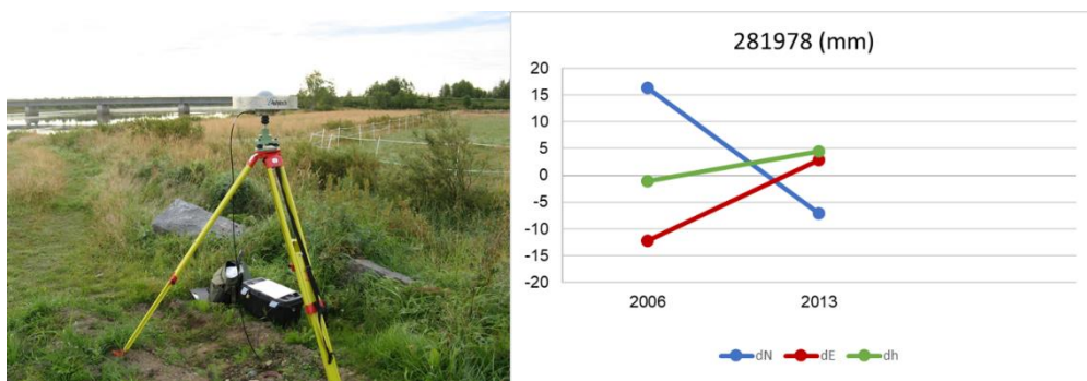
Figure 16: Unstable station excluded from the estimation of general standard uncertainties. Junosuando (281978) is marked with a steelbar in a pipe driven down to bedrock.
