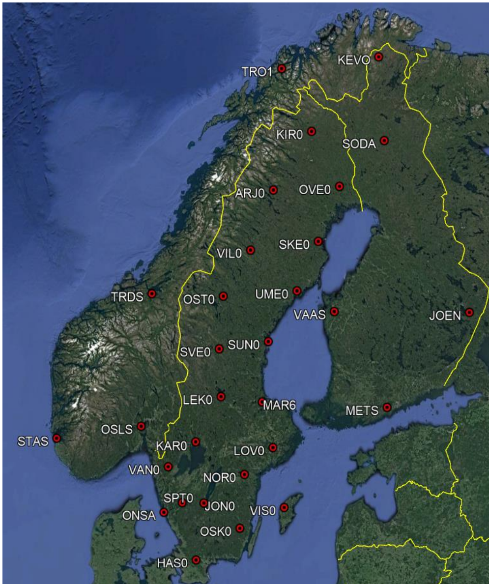
Figure 5: Google Earth map shows the reference stations in Sweden, Norway and Finland which were used in GAMIT daily solutions
