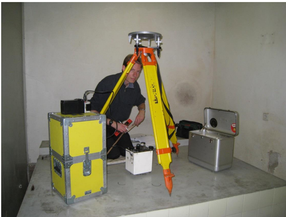
Figure 13: Andreas Engfeldt measuring the gradient in Skopje with LCR G54. Photo: Robert Odolinski.
