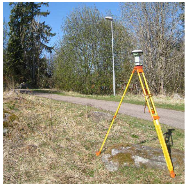
Figure 5: The field measurements with network RTK messages were performed with the GNSS antennas attached to a tribrach on a tripod centred over the points. Photo: Rebecka Lundell.
