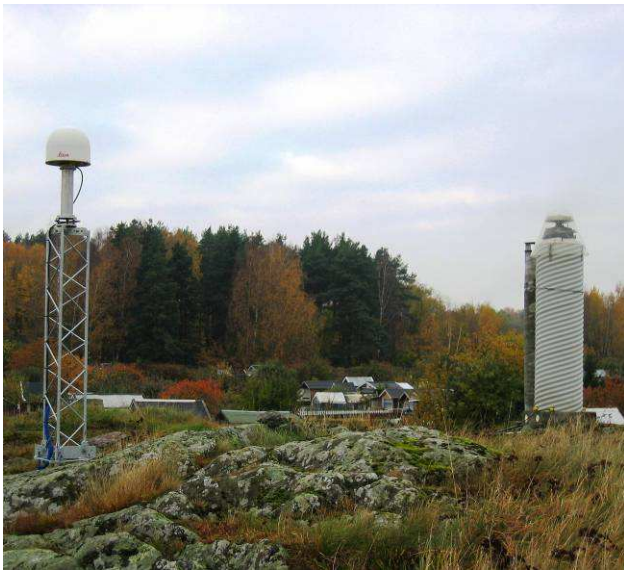
Figure 2: The SWEPOS station Norrköping is an original class A station which has a new steel mast as an additional monument. Photo: Dan Norin.
