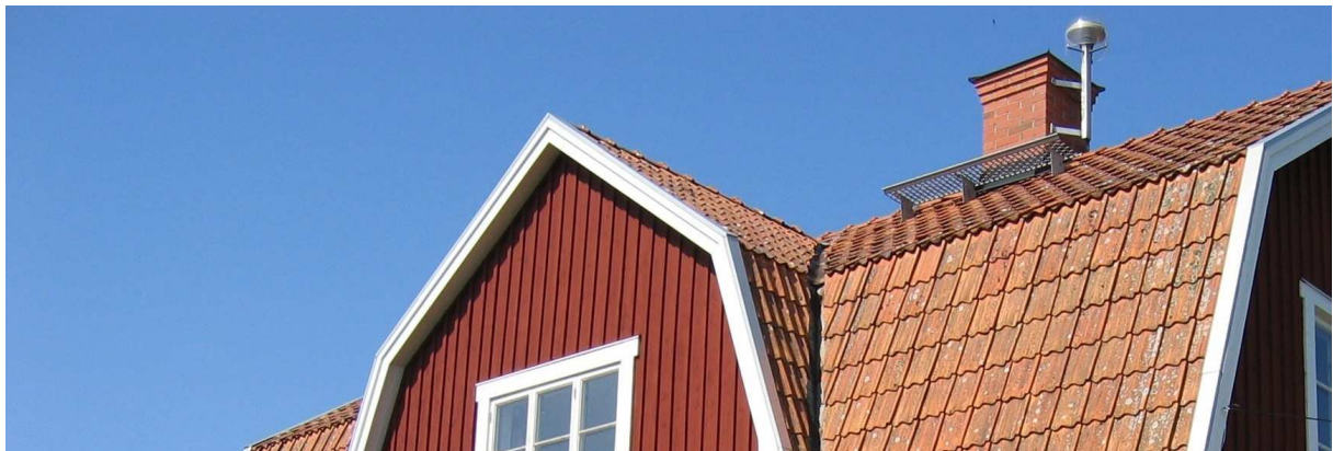
Figure 2-2: Söderboda is a SWEPOS station with a roof-mounted GNSS antenna mainly established for network RTK purposes belonging to Class B.
