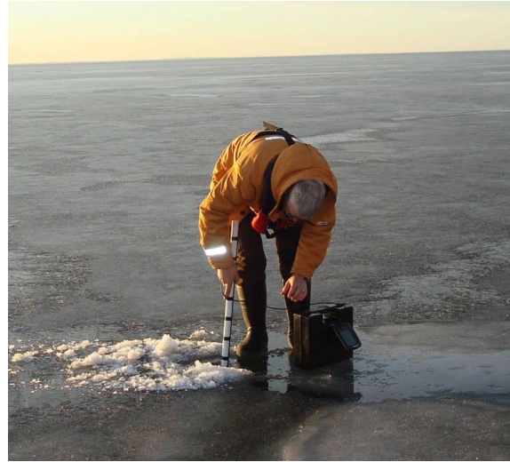
Fig. 5: Measuring depth and ice thickness.
