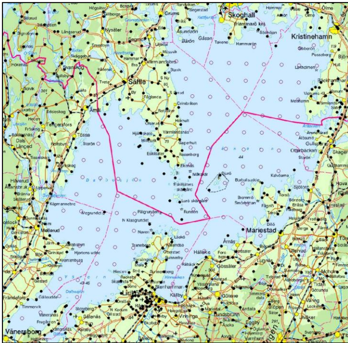
Fig. 2: Old gravity observations around the Lake Vänern (dots) and planned observation spots on the ice (circles).
