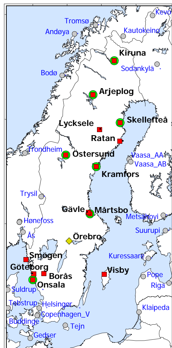
Figure 5: Absolute gravity sites in Sweden (red squares), planned new site (yellow diamond) and sites in neighbouring countries (grey circles). Sites observed every year since 2003 have a green circle as background to the red square.
