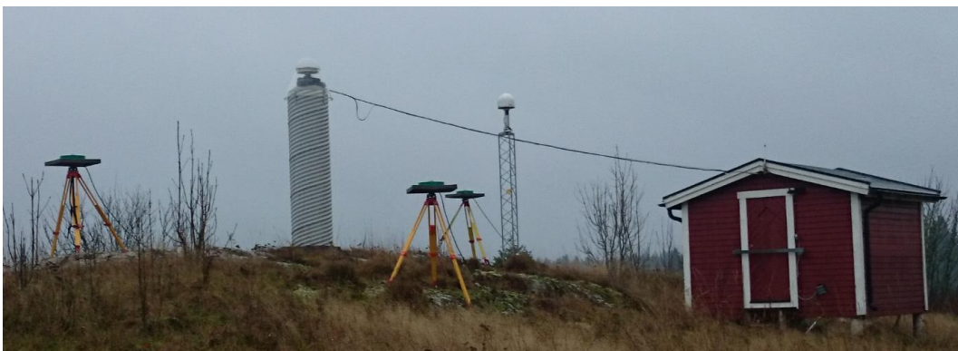
Figure 3.21. The SWEPOS site Vänersborg during a station calibration setup in November 2014. An Eccosorb plate is mounted directly below the choke-ring antenna. Note the typical SWEPOS concrete pillar and the recent steel-grid mast with the LEIAR25.R3 antenna and LEIT radome installed.
