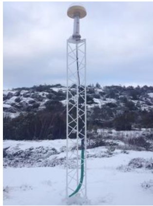
Figure 2.3 The OTT2 mast after being painted white in October 2015. The purpose is to reduce its sensitivity to heating from solar radiation.
