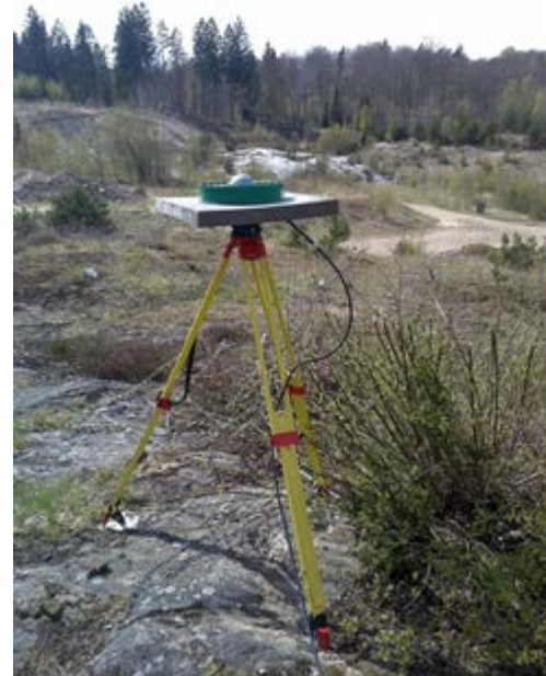
Figure 2. One of the benchmark setups at Hässleholm, 2010. An Eccosorb plate is mounted directly below the choke-ring antenna.
