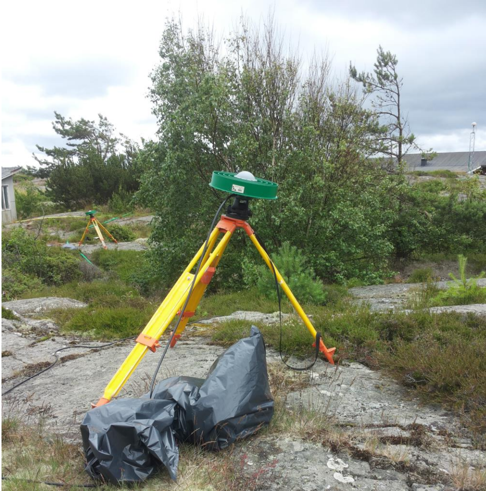
Figure 3.3 The experiment setup at Onsala Space Observatory for determining the consistency of the calibration models from the two calibration facilities, the Bonn group and GEO++. The nearest northern antenna is tilted to west, 13^\circ , while the farther antenna is tilted to east, 14.5^\circ .
